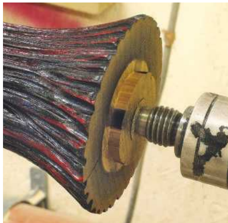
▲ Pic.17 The work is mounted up between centres. You only need enough pressure from the tailstock to drive the work. The speed of the lathe should ideally be around 1000rpm
